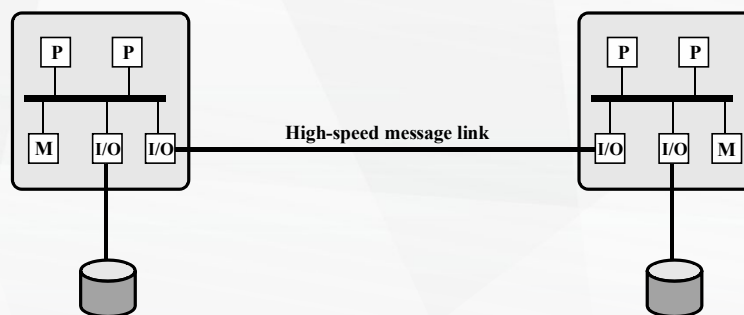
(a) Standby server with no shared disk
